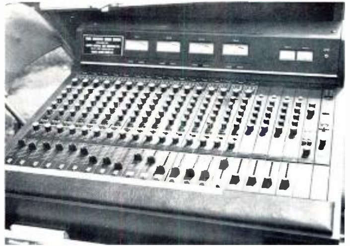
16-in/4-out console with each input switchable to any of four line, two echo, and four monitor outputs. Each input also has equalization controls.
