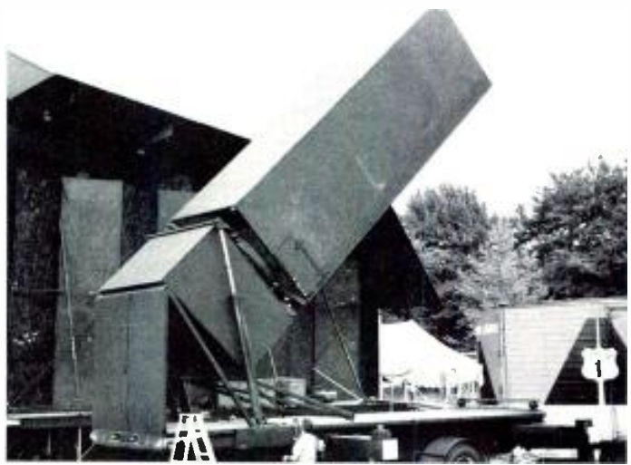
Still weather-protected, the left speaker tower is raised from the truck bed into its upright position.
